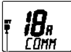
Appears when the lock function is in use.
